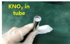
Fig. 1. the physical role of \text{KNO}_3 filler in the swaging process.
