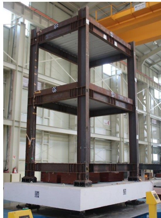
Fig. 1. Base-isolated frame structure for shaking table tests
