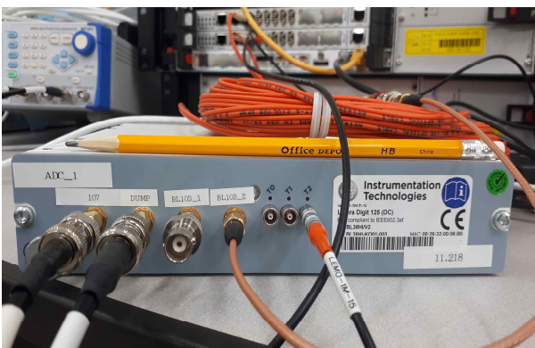
Fig. 4. Libera Digit 125 for beam current monitoring
