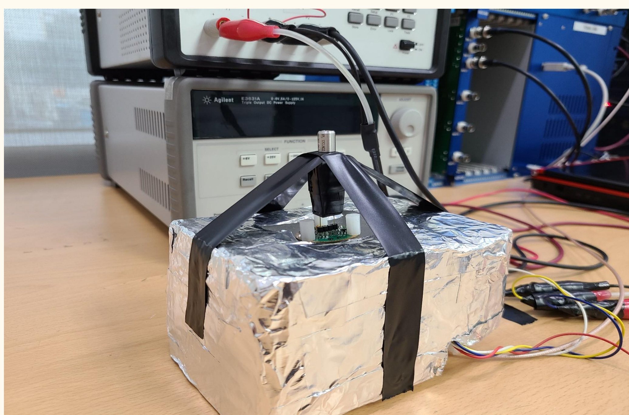
Fig. 1. Experiment setup of a ^{252}\text{Cf} source, EJ276G scintillator and SiPM
