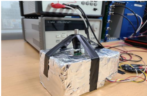
Fig 2. Experimental setup of a ^{252}\text{Cf} source, EJ276G scintillator and SiPM
