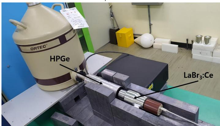
Fig. 1. LaBr<sub>3</sub>:Ce scintillator and HPGe detector deployment
