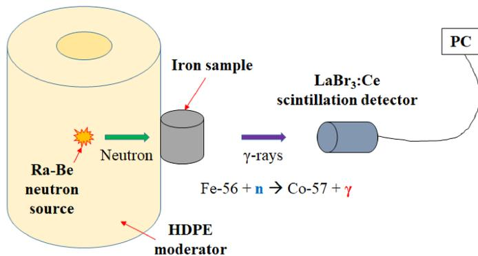
Fig. 2. Setup for FNAA on an iron sample
