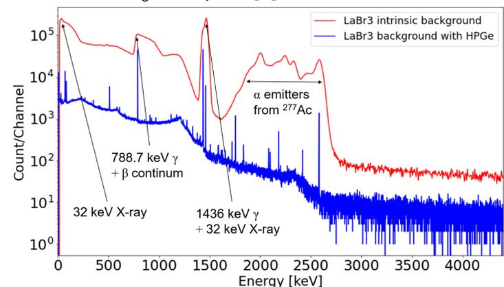
Fig. 3. The background spectra measured with LaBr<sub>3</sub>:Ce and HPGe detectors
