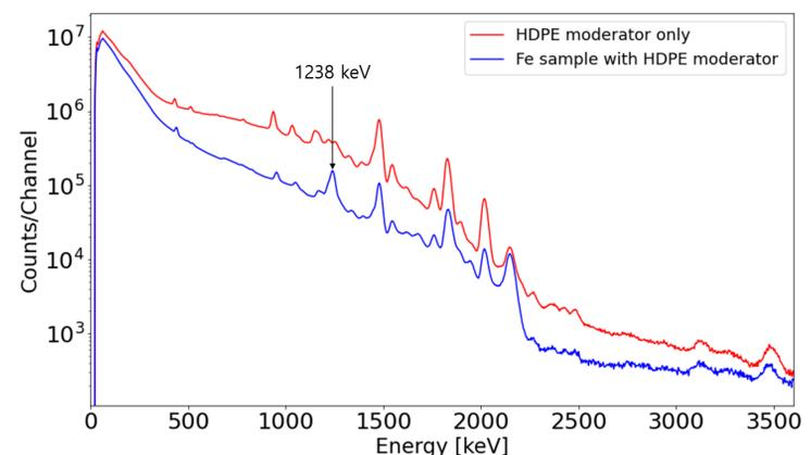
Fig. 4. Spectra of  $\gamma$ -rays from iron sample irradiated with Ra-Be neutron source
