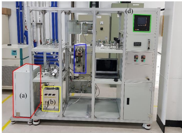
Fig. 1. Layout of the AMSB apparatus: (a) dryer, (b) vapor generator, (c) test section with a furnace and (d) vapor analyzer
