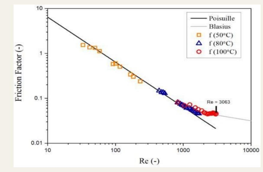
The experiment was carried out until the Reynolds number is 3063. As figures shows, the value of differential pressure increases linearly following Reynolds number.
