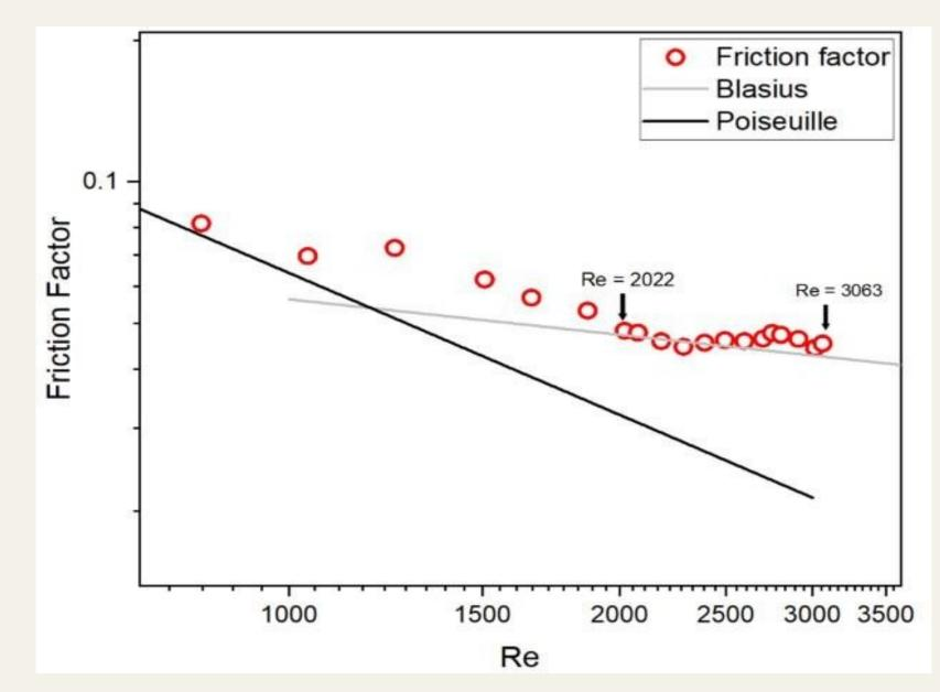
As figure shows, around Reynolds number is around 1000, it looks like transition region has started. Accordingly, the experimental friction factor value matches with Poiseuille friction factor and Blasius friction factor. The maximum error of the measured friction factor is 15%.
