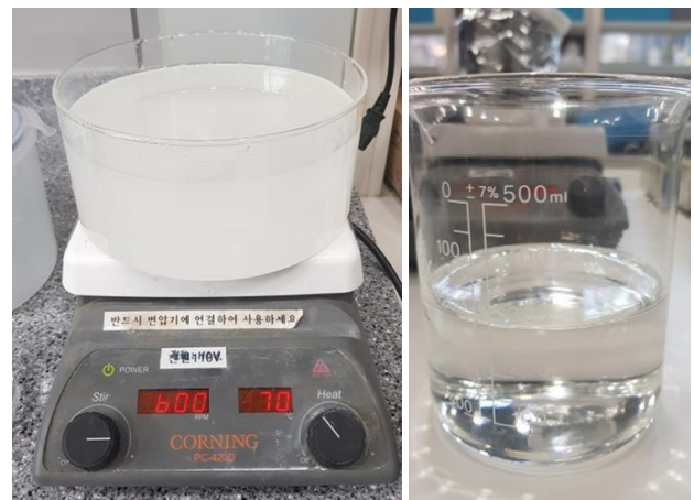
Fig. 1. Glyceline manufacture process and result
