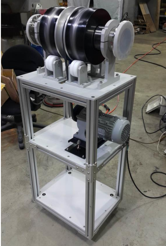
Photo. 1. Fabricated beam wobbler in test operation.
