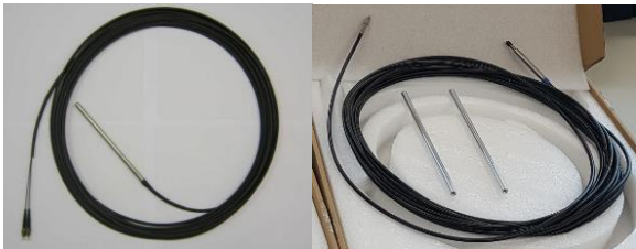
Fig. 2. An existing (Left) and newly developed (Right) optical fiber-based scintillation detector
