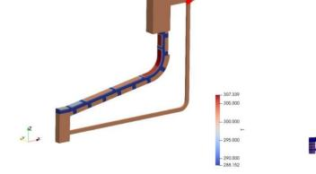
• The mesh consists of about 50,000 fully hexahedral cells and is divided into three parts: flow, catcher and stud.
