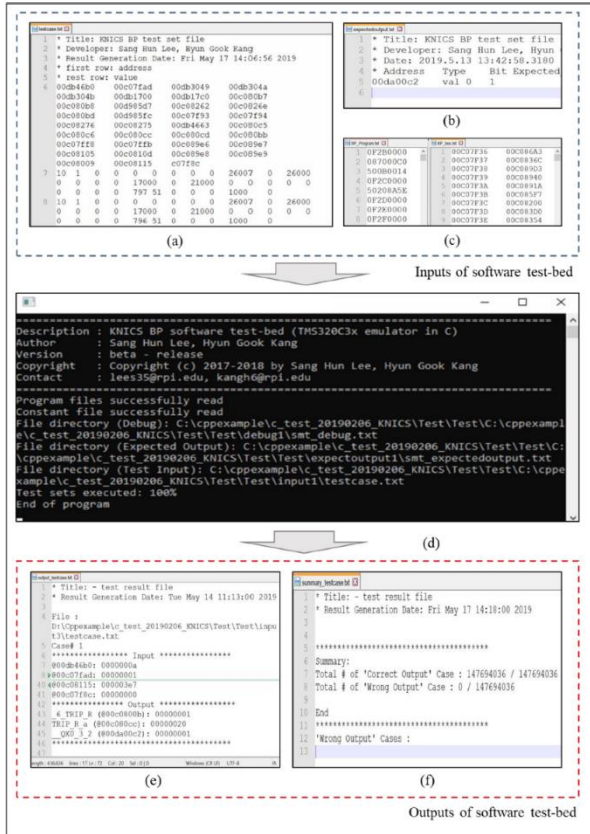
Fig. 4. Test results of the case study for BP pressurizer-pressure-low trip logic: (a) Test case file, (b) Expected output file, (c) Program file, (d) Screenshot of simulation-based test-bed execution, (e) Test result file, (f) Test summary file.
