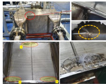
Fig. 1. Photos of the serious leak on the recuperator (on top) and inspection results of the recuperator core (on bottom)
