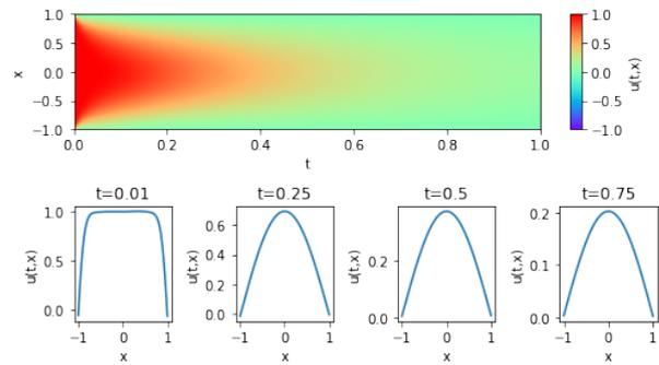
Figure 3 PINN Analysis result (Time dependent heat conduction equation)
