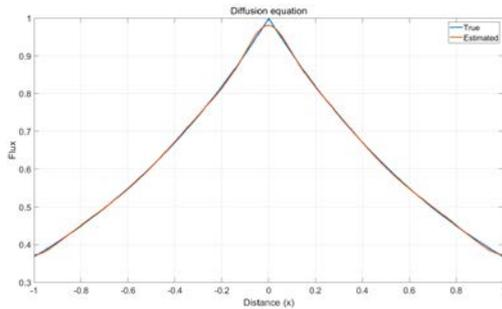
Figure 2 PINN analysis result (Diffusion equation)
