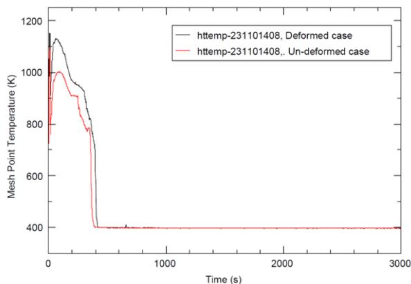
Fig. 2. Comparison of cladding temperature between deformed case and un-deformed case
