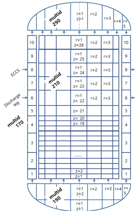
Fig. 1. Nodalization of RV by multid components
