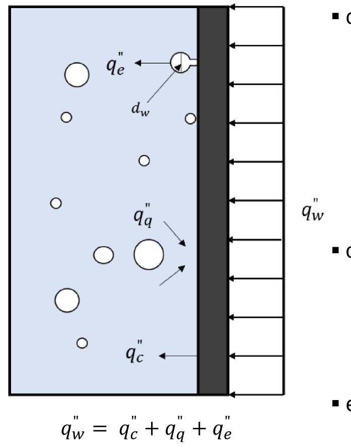
• convective heat flux  $(q_c)$ •  $q_c'' = h_c (T_w - T_l)(1 - A_b)$ •  $A_b = \min\left(1, K \frac{N_w \pi d_w^2}{4}\right)$ • K = 4.8 exp $\left(-\frac{\rho_l c_{p,l}(T_w - T_l)}{800 \mu c}\right)$
