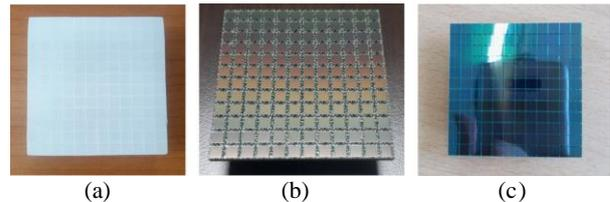
Fig. 1. Stilbene scintillator array ( $12 \times 12$  pixels of  $4 \times 4 \times 20$  mm<sup>3</sup> each) (a), C-series SiPM array ( $12 \times 12$  pixels of  $3 \times 3$  mm<sup>2</sup> each) (b), and a self-developed J-series SiPM array ( $12 \times 12$  pixels of  $4 \times 4$  mm<sup>2</sup> each) (c).
