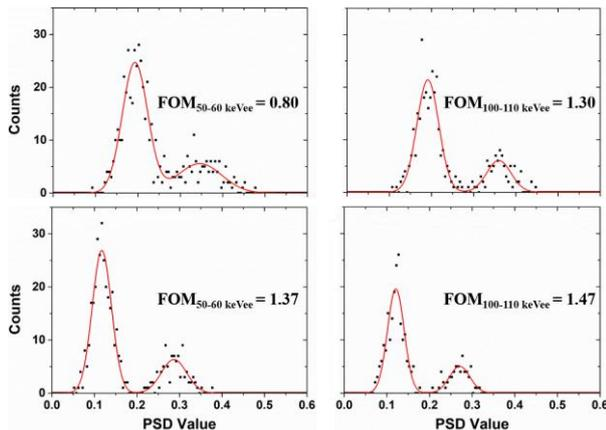
Fig. 4. FOM values in a low energy range for a single-pixel PSD distribution obtained from each C-series (top row) and J-series SiPM-Stilbene array sensor module (bottom row).
