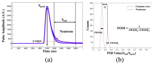
Fig. 3. Illustration of the PSD method (a) and FoM evaluation method (b).
