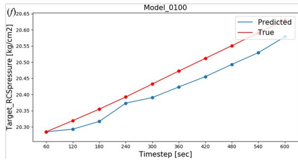
Fig 4. Prediction results of model #4, where only charging flow control valve open signal is on (True: actual value, Predicted: predicted value). (a) and (b): PZR level, (c) and (d): RCS loop#2 average temperature, (e) and (f): PZR pressure.
