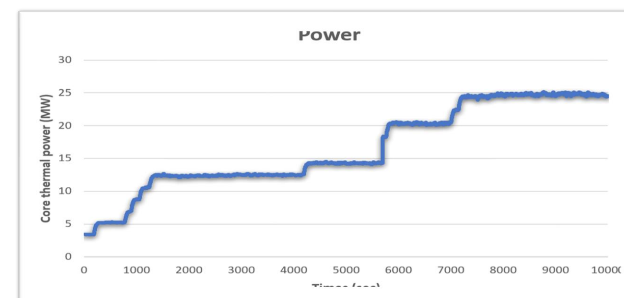
Fig. 4. HANARO core thermal power with time change.
