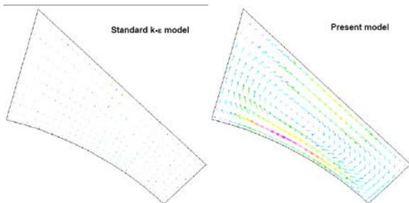
Figure 1 Secondary flow with the standard k- $\epsilon$  and the quadratic k- $\epsilon$  model
