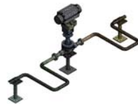
Fig.2 Mesh model of HCS and isolation valve
