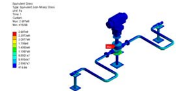
(b) Combined thermal and seismic loads
