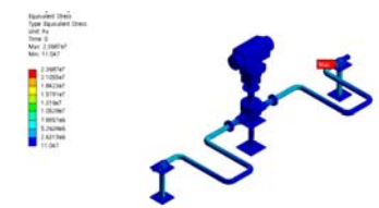
(c) Combined pressure and seismic loads
