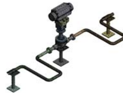
Fig. 2. Mesh model of HCS and isolation valve
