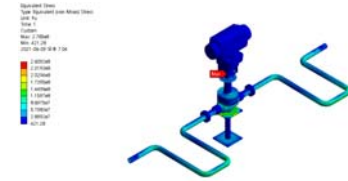
(a) Combined thermal and pressure loads
