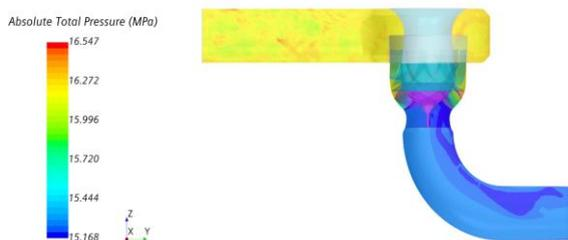
Fig. 3. Pressure distribution on the impeller center section plane.
