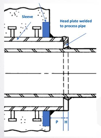
Originally, the penetration in the pool was a **projection type**.
