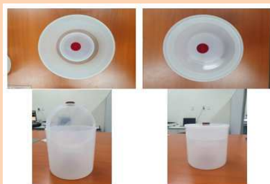
Fig 2. Check Source position at each distance (0 cm top left, 3 cm, 7cm, 14 cm Clockwise)
