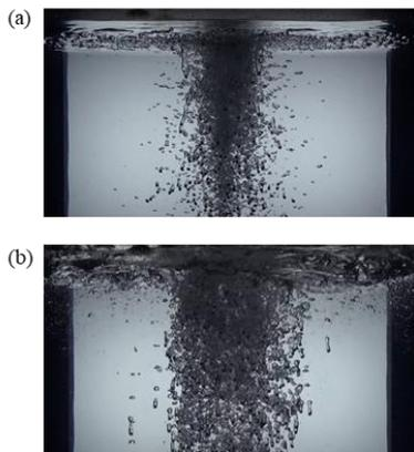
Fig. 3. Particle falling images (a) without and (b) with heating
