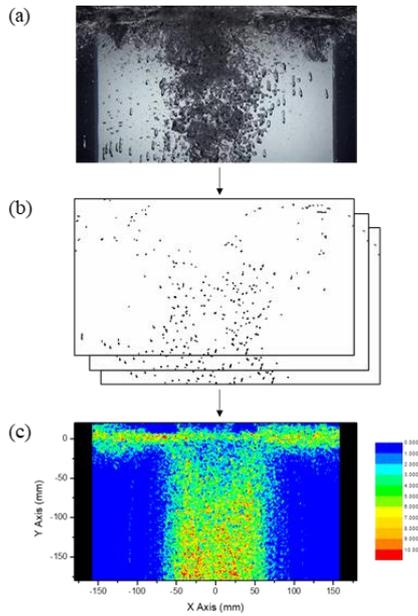
Fig. 2. Method to obtain dispersion of particle jet
