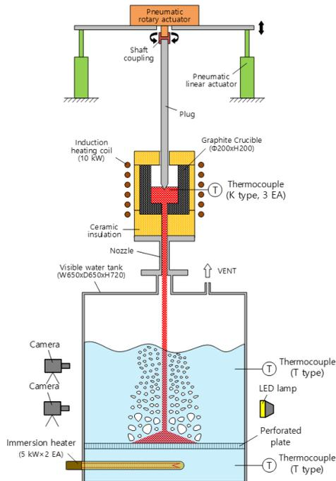
Fig. 1. Experimental schematic of DEFCON-S
