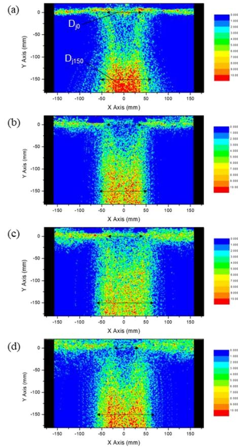
Fig. 4. Dispersion of particles within initial 2 s with (a) non-heated cylinder, (b) 500°C heated cylinder, (c) 800°C heated cylinder, and (d) 800°C heated sphere particles
