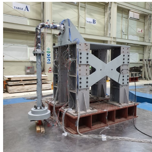
Fig.1 Setup of excitation test using shaking table
