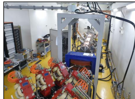
Figure 6. Overview of the 1 MeV/n RFQ accelerator, KOMAC
