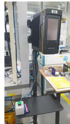
Fig. 4. Remote controller of the remote fastening system
