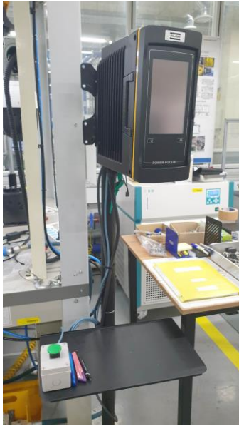
Fig. 3. Remote controller of the remote fastening system
