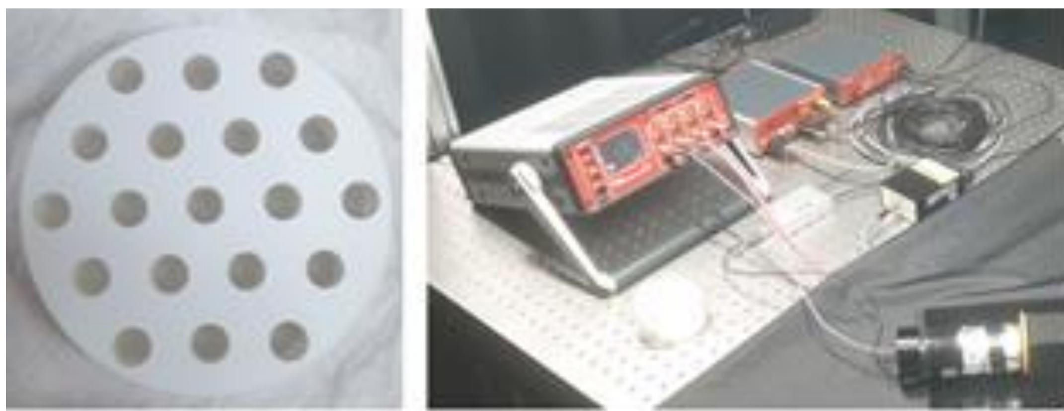
Fig 1. The scintillator with nineteen holes (left) and the experimental composition (right)
