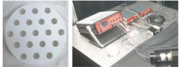
Fig. 1. The scintillator with nineteen holes (left) and experimental composition (right)
