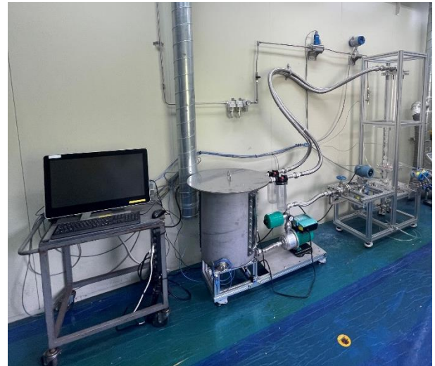
Fig. 2 Pressure drop test facility
