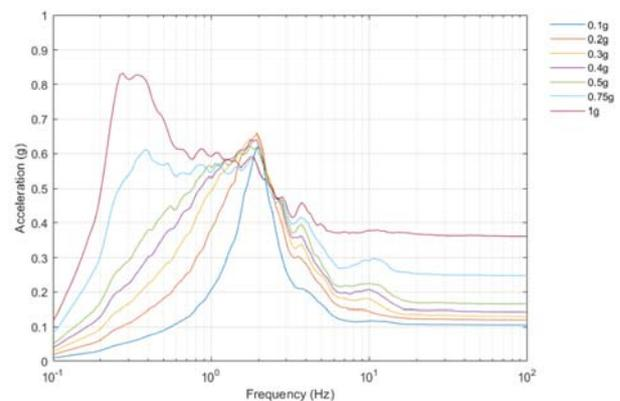
Fig. 2. FRS on auxiliary building 78 ft. in the isolated NPP
