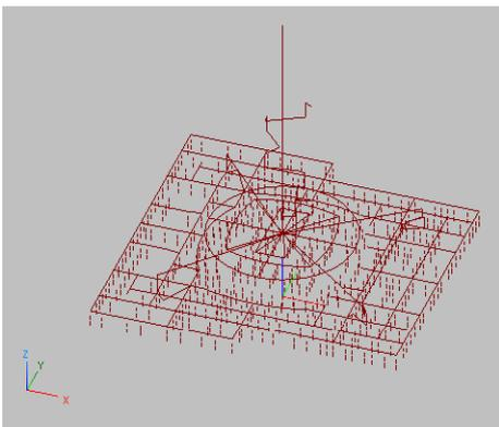
Fig. 1. Numerical model of the isolated NPP
