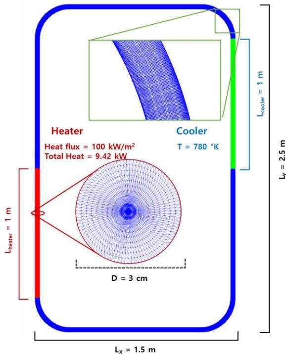
Fig. 1. A schematic of natural circulation loop outline for OpenFOAM simulation
