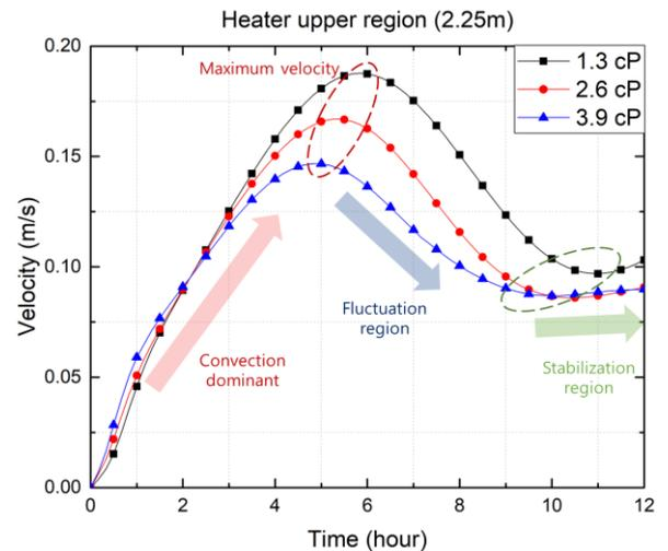
Fig. 3. Velocity profile of internal flow at heater upper region over time
