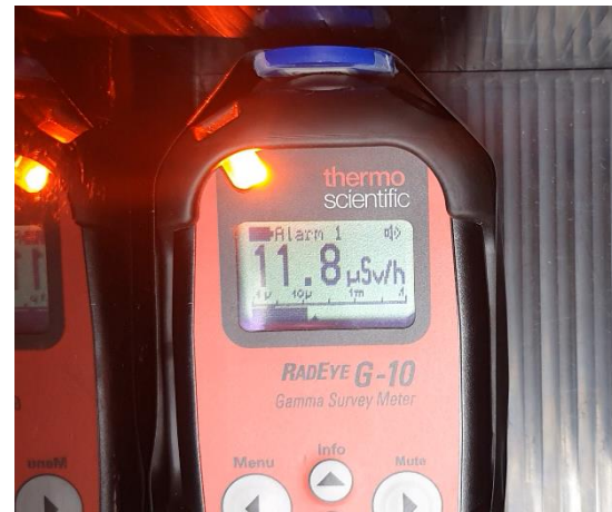
Fig. 3. Experimental setup to measure dose-rate with a survey meter.
