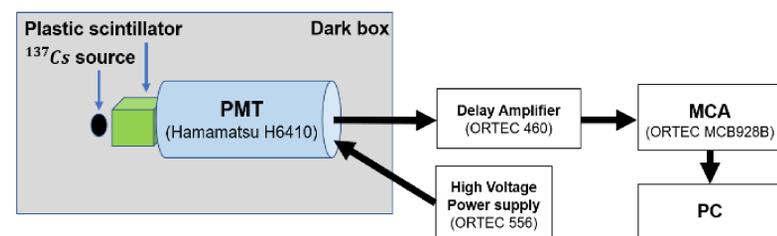
Figure 3. Measurement system for scintillation light output.
