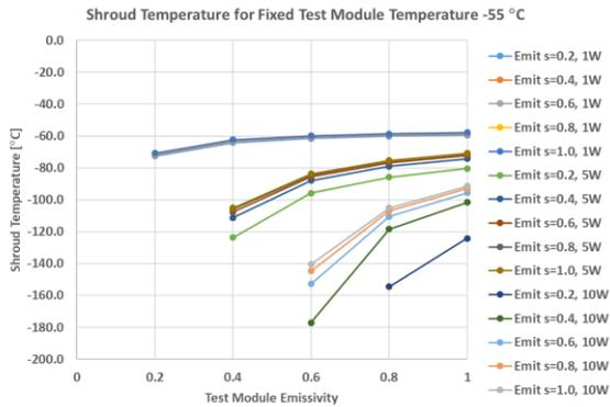
Fig. 2. Shroud temperature for fixed DUT temperature -55 °C depending on DUT heat and emissivity.
