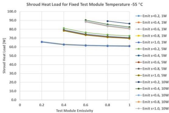
Fig. 3. Heat load on the shroud for fixed DUT temperature -55 °C depending on DUT heat and emissivity.
