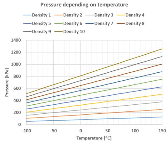
Fig. 5. Nitrogen gas pressure depending on density and temperature.
