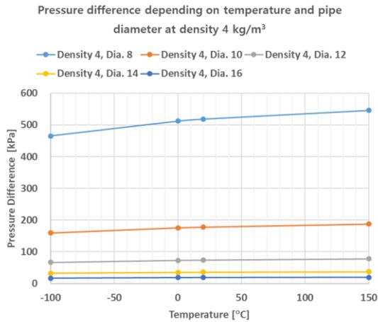
Fig. 7. Pressure drop through the shroud depending on the pipe diameter and temperature at nitrogen gas density 4 kg/m<sup>3</sup>.
