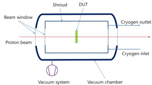
Fig. 1. The schematics of the space simulation chamber.
