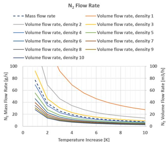
Fig. 6. Nitrogen gas mass and volume flow rate.
