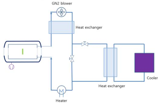
Fig. 4. Schematics of the temperature control system.
