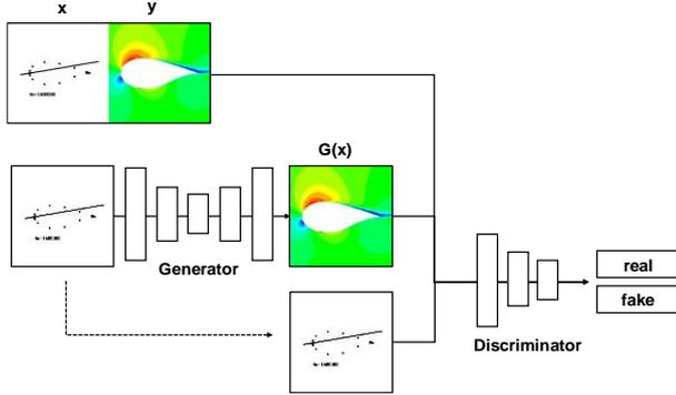
Fig. 3. The flow chart of pix2pix for airfoil flow field prediction
