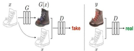
Fig. 2. Structure of pix2pix [3]
