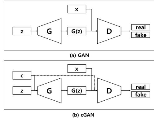
Fig. 1. architecture of GAN and cGAN.
