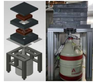
Fig. 1. Schematic view (left) and configurations (right) of measurement system consisting of HPGe detector, LN 2 dewar, lead bricks and 1 cm thickness copper box.
