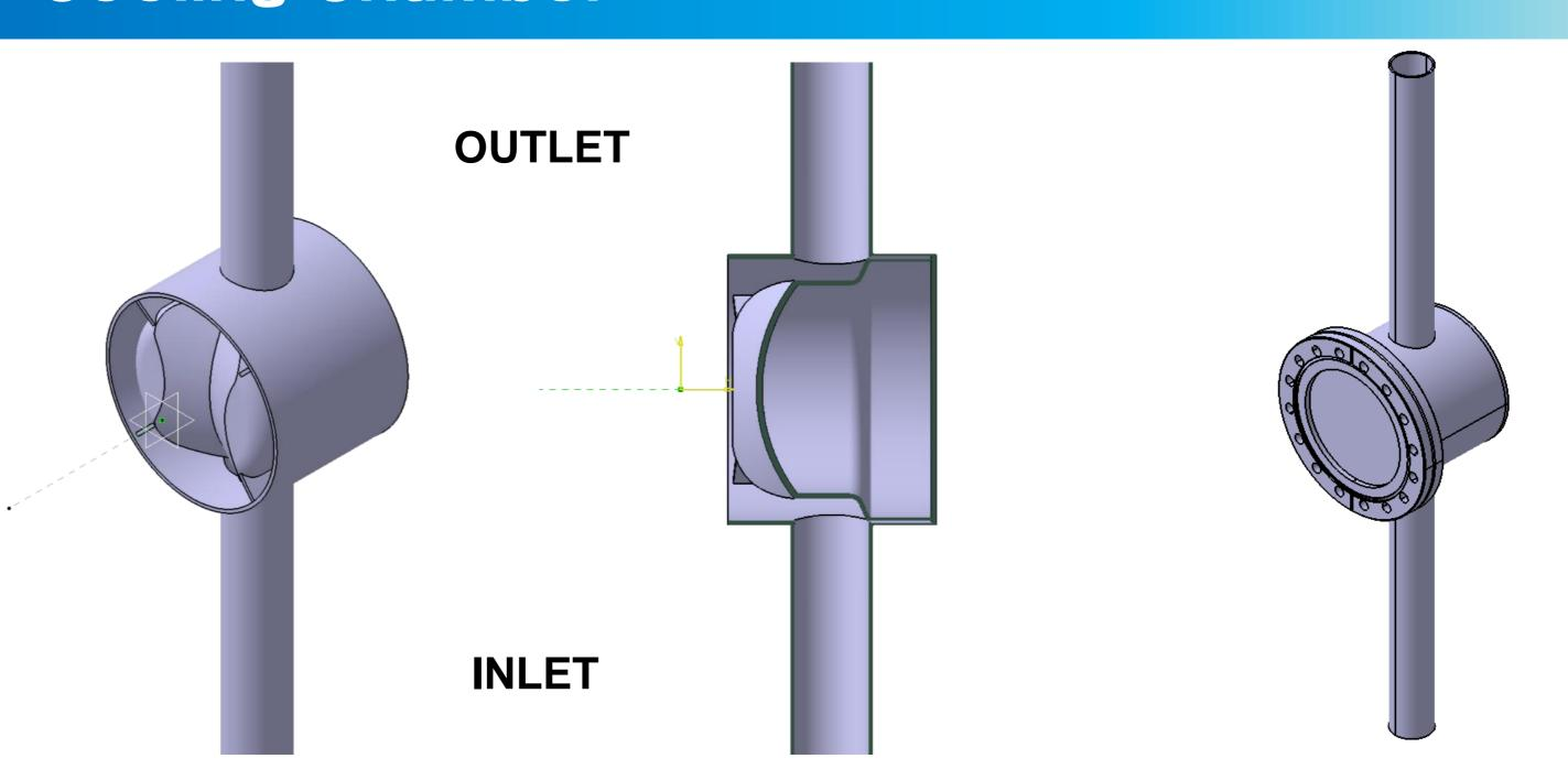
• The diameter of the proton beam incident on the target is assumed to be 3 cm, giving the thermal load of 1.4  $MW/m^2$
