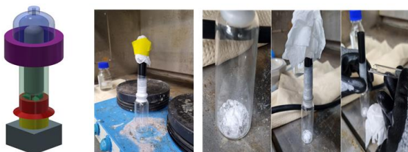
Fig. 4. Prototype of crushing device and testing results
