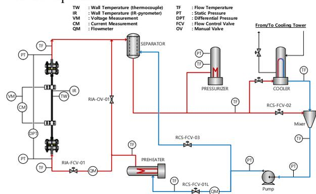
Fig. 1. Schematic of the THERA test facility
