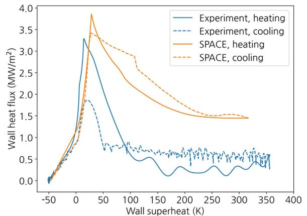
Fig. 5 Boiling curve
