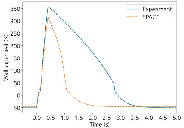
Fig. 3 Wall superheat with time
