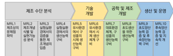
Fig. 2. Manufacturing Readiness Level (MRL) for Mo-99 production.
