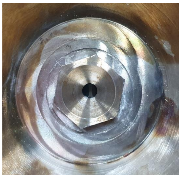
Fig. 2. Experimental specimens were observed through a diamond window view cell.
