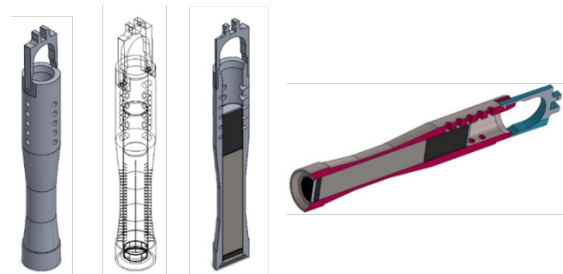
Fig. 2. Final 3-dimensional model of the SiC-NTD irradiation basket
