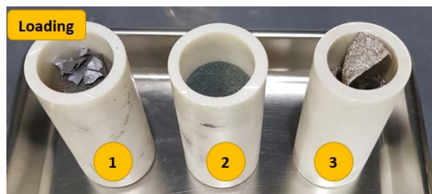
Fig. 2. Loadings: raw material(No.1), atomized powder(No.2) and crushed ingot(No.3)
