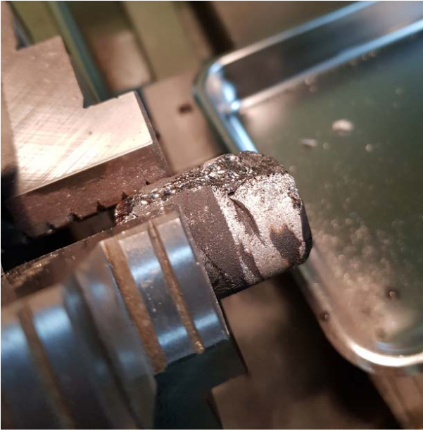
Fig. 5. The lathe machining result of the No.2 U_3Si_2 ingot
