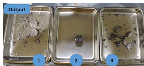
Fig. 3. Fabricated U_3Si_2 ingots: raw material(No.1), atomized powder(No.2) and crushed ingot(No.3) loadings
