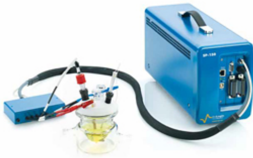
Fig. 2. Electrochemical measurement instruments to evaluate the hybrid composite electrodes (SP-200, biologic, France)
