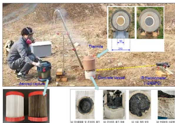
Fig. 1. Photos of molten iron-concrete reaction test (lower left: filters before and after aerosol capture, lower right: iron and concrete after reaction)
